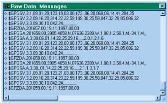
normal operation of the window. Note that scrolling back, thus freezing the screen, allows the data in the window to be selected and copied. Data copied may then be pasted into any other application such as Notepad, a word processor or an e-mail editor.
