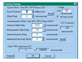
For high accuracy timing synchronized to UTC the Epoch, Offset and Intentional Early Offset controls are normally set to zero (0) and the Antenna Cable Delay, Measurement Cable Delay and Internal Receiver Delay controls are set as accurately as possible.
